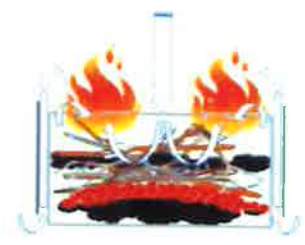
Ring of Fire Biochar Kiln® Airflow and flames - Coaster-flow, air from the top keeps embers contained and flame reignites flow.
