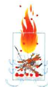
Burn Barrel Airflow and flames - all from the bottom, transports embers out of the barrel.
