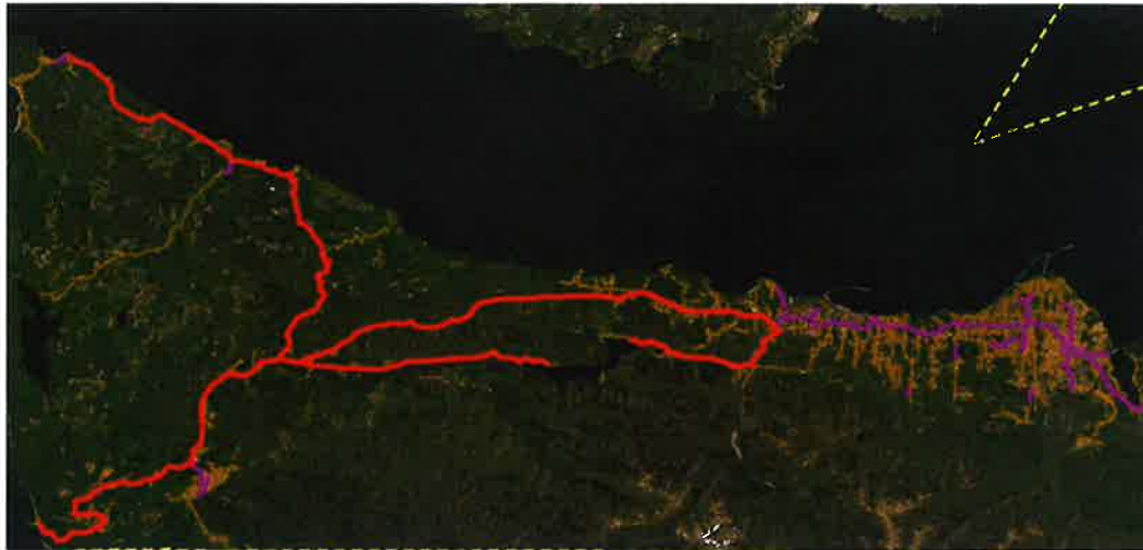
Figure 8. Proposed Fiber Optic Infrastructure Scenario (Middle Mile Build Scenario)
