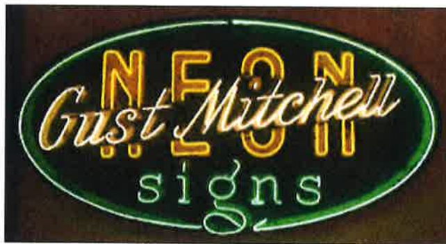
Border tubing is the exterior perimeter of neon tubing that frames the sign. Historically fabricated with neon, flexible, LED-lit tubing offers another option for illuminated borders. Photo taken at the American Sign Museum.
