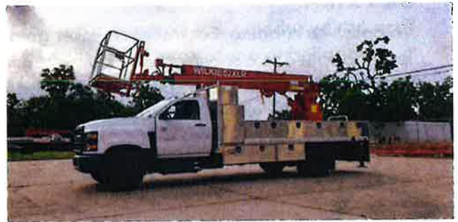
Cranes, such as this Wilkie 52XLR, are an essential tool for sign installation. Operators of cranes with a capacity of more than one ton are required to be certified by a federally approved school or facility. Photo provided by Wilkie Mfg. Co. (Oklahoma City)
